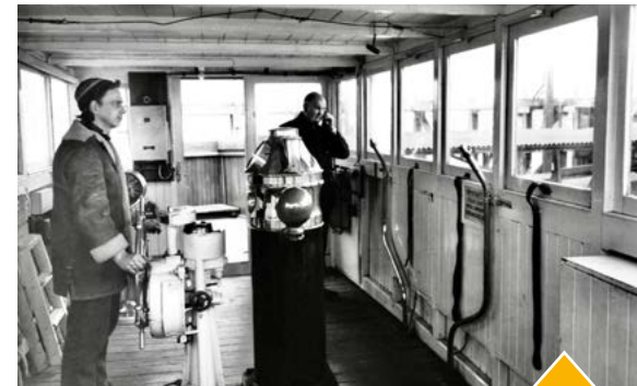
The Captain and Helmsman on the bridge. The two speaking tubes to the engine room are seen below the windows.
